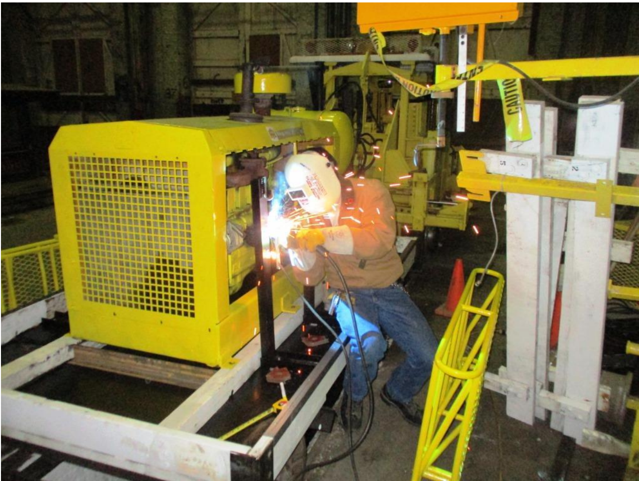
Kyle welds a cross-brace on the mounting brackets that Alan designed for the Nolan Flat Car on the air-compressor to provide more stability
