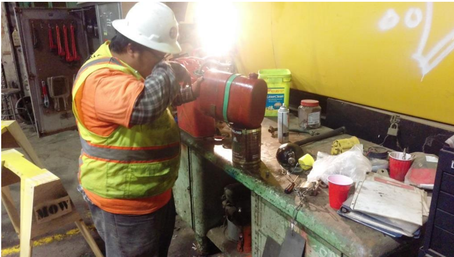
Anthony drains the old rotten fuel out of the derrick car's gas-tank
