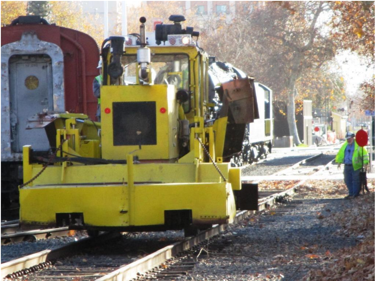
Frank acts as brakeman for the ballast regulator which returned to town under its own power
